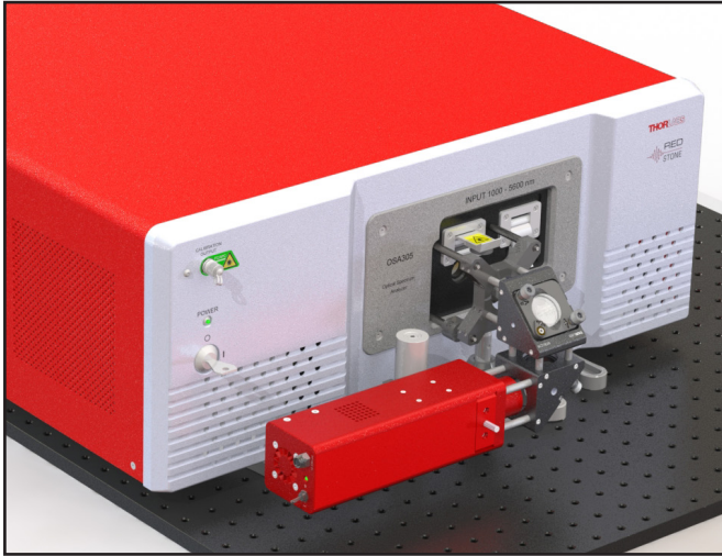
Figure 5: An example free-space setup suitable for a broadband divergent source, which includes the Thorlabs SLS203L Stabilized Free Space light source. The source is kept at a short distance from the OSA to minimize input losses.
