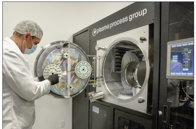
Ion Beam Sputtering Chamber for Ultrafast Optics in Thorlabs' Headquarters in Newton, NJ
