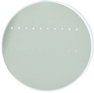
The photograph above is a protected aluminum-coated mirror after LIDT testing. In this particular test, it handled 0.43 \text{ J/cm}^2 (1064 nm, 10 ns pulse, 10 Hz, \varnothing 1.000 \text{ mm} ) before damage.
