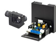
Click to Enlarge GVS011 Silver-Coated Galvo Mirror Assembly and Driver Board
