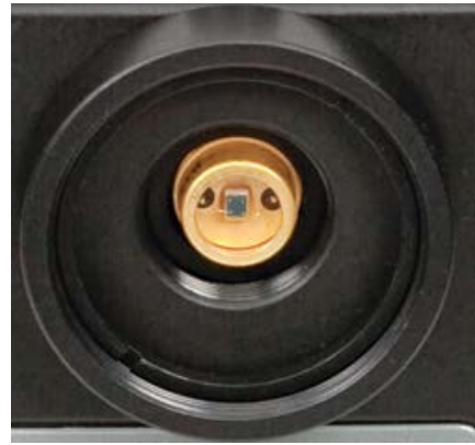
A close up picture of the front of the PDA10A photodetector. The internal SM1 threading on the SM1T1 adapter and internal SM05 threading on the photodetector housing can be seen in this image.
